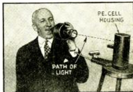
A simple device for speaking on a light beam being demonstrated by Dr. J. B. Kramer. It consists of only a battery, flashlight and microphone!
