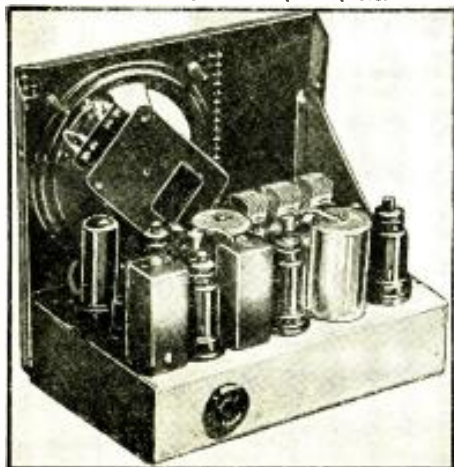
The rear of the receiver chassis showing the compact mounting of tubes, coils, etc.
